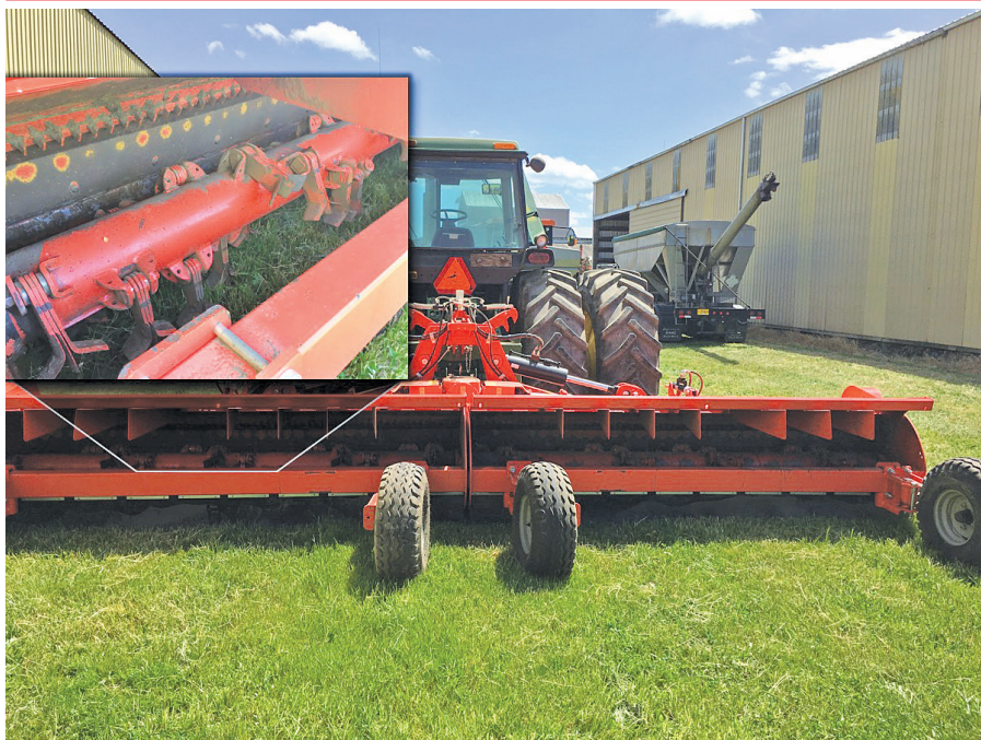
FIGURE 3 Flail choppers shred the residual straw to ensure decomposition and minimal effects after seed harvest.
