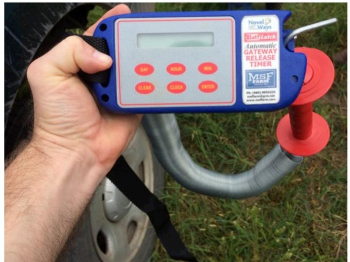
**Figure 2.** Technology that automatically releases a gap in the electric fence can be a great labor saving device when using timed grazing.
