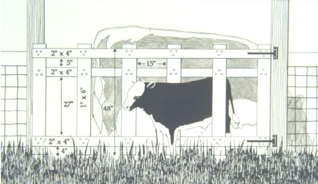
**Figure 3. A creep gate that uses a single strand of electrified wire elevated at approximately 50" (note wire and insulator on top of post in foreground). Calves on this farm creep grazed oats while cows refused to travel under the wire and were maintained on bermudagrass hay. Courtesy of Scott Sell, County Extension Agent in Screven County, GA.**
