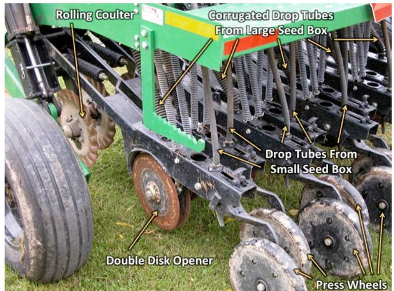
**Figure 2.** Parts of a no-till drill.
