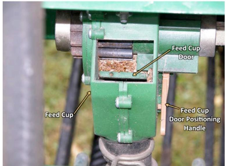
**Figure 1.** This feed cup (under each seed box) is full of seed from the previous use.
