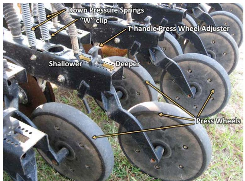
Figure 3. Parts important to ensuring proper opener/seeding depth.
