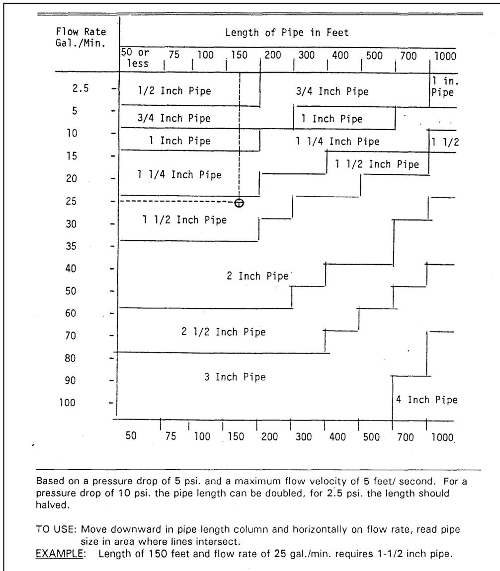
Figure 3: Recommended Size for PVC or Plastic Pipe
