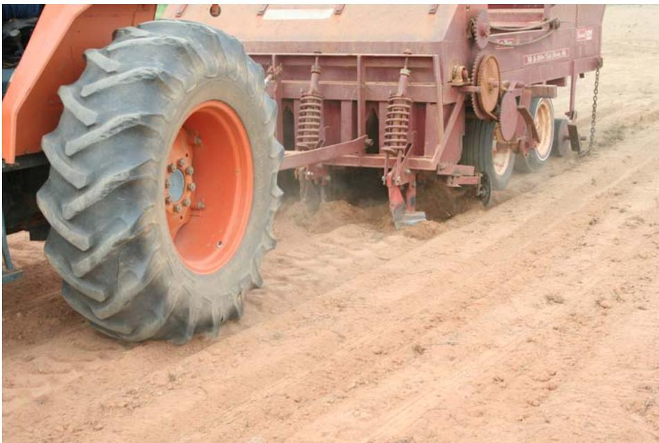
**Figure 8.** A commercial sprigging machine simultaneously creates a furrow, drops sprigs, covers and firms the furrow, and smoothes the soil.
