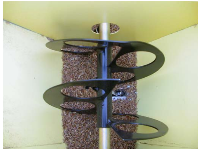
Figure 1. A seed box agitator is necessary to prevent the fluffy seeds of some NWS grasses from clogging openings in the seed box.
