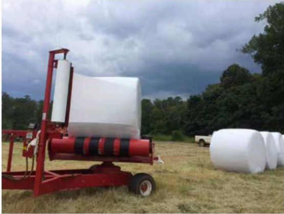
Figure 1. Examples of two basic categories of baleage wrappers: individual bale wrapper on a trailer platform (left) and an inline bale wrapper (below).
