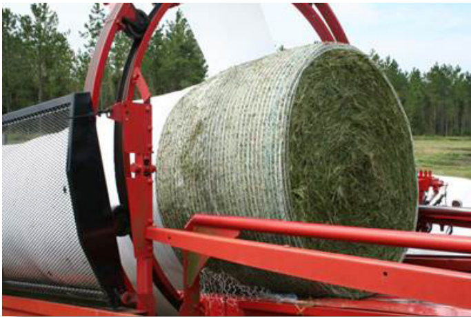
Figure 2. Picture of in-line baleage wrapper. Photo credit: Dr. Dennis Hancock, University of Georgia.
