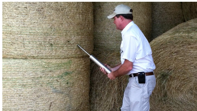
Figure 3. Sampling a lot of hay bales using a Colorado hay probe.
