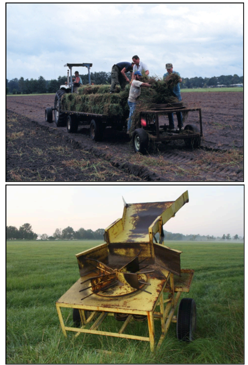
Figure 2. Square bales of bermudagrass tops are being scattered over a prepared seedbed (top) using a ground-driven tops spreader.
