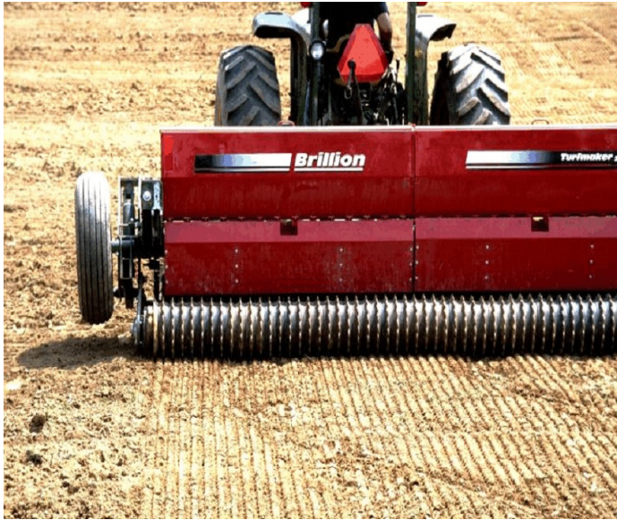
Cultipacking-seeder planting into a firm seedbed.
