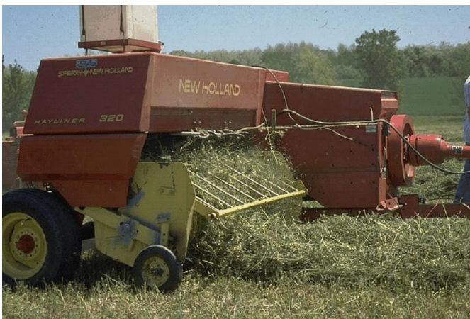
Hay preservative being applied to alfalfa hay as it is being baled.
