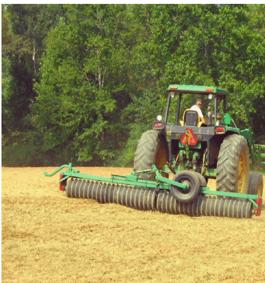
A cultipacker can help firm the soil prior to planting.
