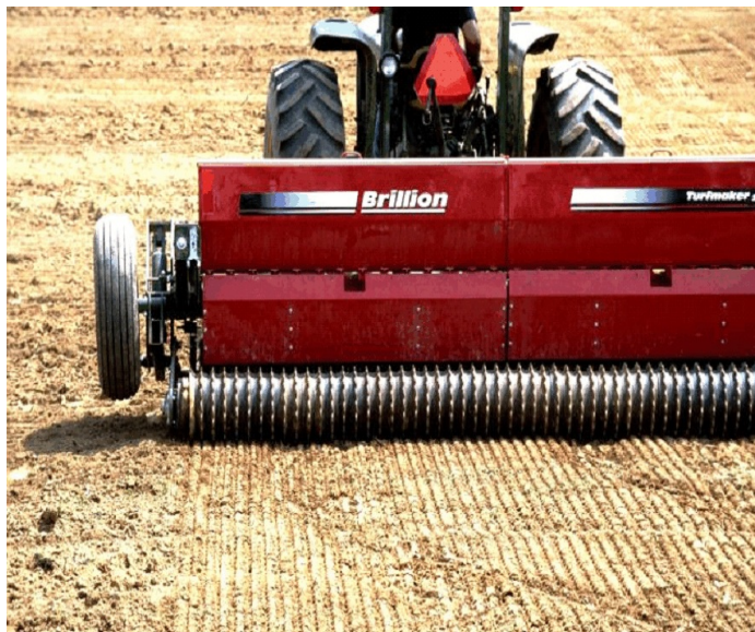
Cultipacking-seeder planting into a firm seedbed.
