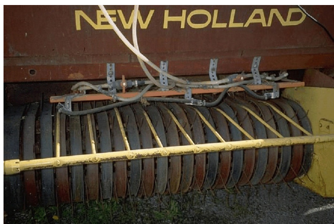
Hay preservatives can cause excessive corrosion on equipment.
