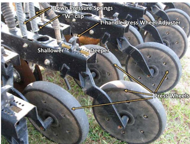
Figure 3. Parts important to ensuring proper opener/seeding depth.
