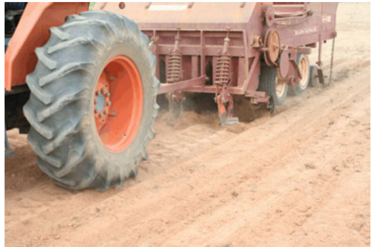
Figure 8. A commercial sprigging machine simultaneously creates a furrow, drops sprigs, covers and firms the furrow, and smooths the soil.
