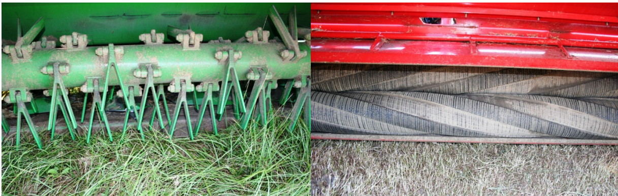
Figure 2. The two conditioner styles: impeller or flail-type (L) and roller-crimper (R).
